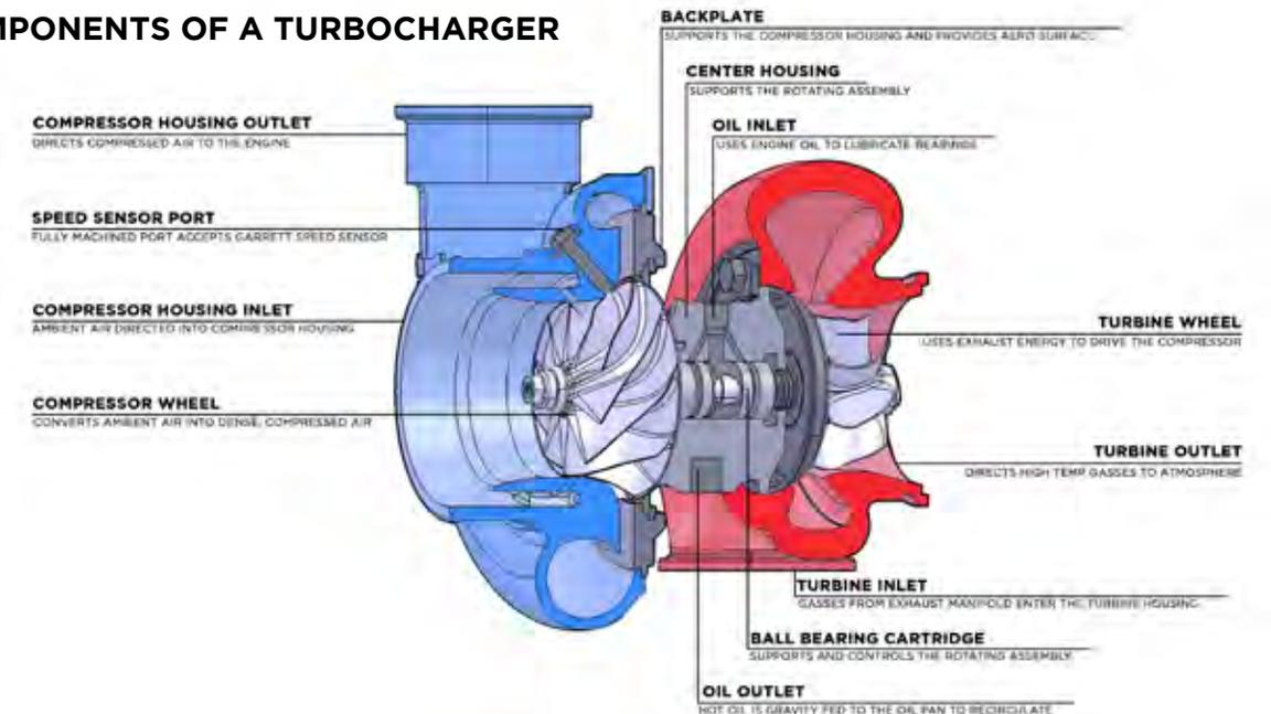
Ball bearing innovation began as a result of work with the Garrett Motorsports group for several racing series where it received the term the “cartridge ball bearing”. The cartridge is a single sleeve system that contains a set of angular contact ball bearings on either end, whereas the traditional bearing system contains a set of journal bearings and a thrust bearing.
