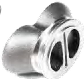
**Divided Vband Inlet Adapter:** The Garrett divided V-band adapter is for enthusiasts that are fabricating divided exhaust manifolds. This adapter mates perfectly with GT/GTX 30 and 35 divided Vband turbine housings and has two 2" recessed orifices that feed into the flange.
